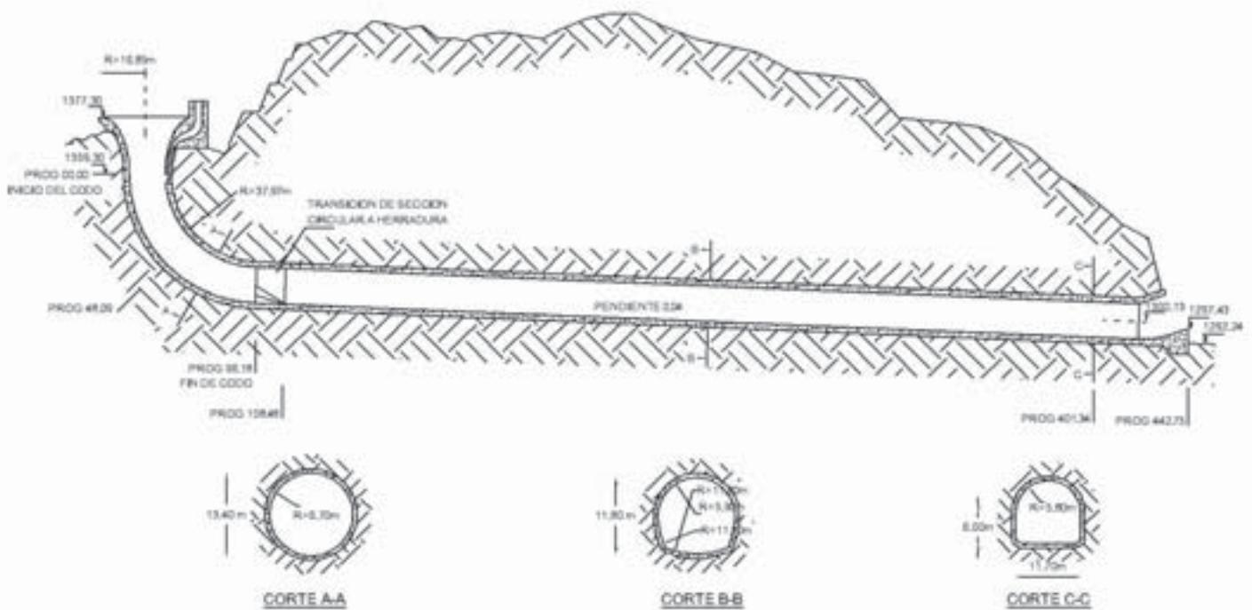
**CORTE ESQUEMATICO DE LA TUBERIA FORZADA A CENTRAL CACHEUTA
